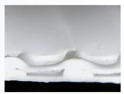
FIG.2 200X magnification of a seal performed with traditional hot-die cutting machine. Alveolar sheet in PP 3 mm thick e weight of 600 gr / m2.
