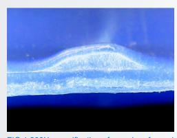
FIG.1 200X magnification of a seal performed with SIGNO.
