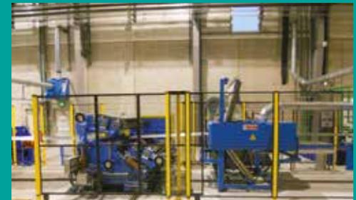
Horizontal Chemical Coater and IR Chemical dryer
