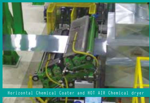
Horizontal Chemical Coater and HOT AIR Chemical dryer
