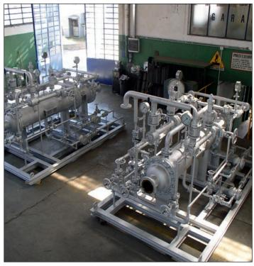
The most frequent applications are in energy and production industries. Furthermore, countless chemical and petrochemical plants adopt ejectors for keeping the vacuum necessary for processing fractional distillation, crystallization, drying, deaeration, filtration and impregnation. Particularly, all the plants for deodorization and fatty acid treatment lately built are fitted with steam jet thermocompressor ejectors which allow very low final residual pressures.
