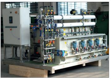
We studied, built, tested and patented this new mixed system that combines other three processes: a double desalination system of Reverse Osmosis, a Chemical Process and a Solar Evaporation Point, thereby obtaining the maximum possible production of desalted water with an almost zero discharge of brackish water.
