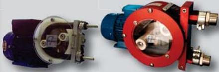
*Production of pumps for industrial processes with aluminum or engineering plastic pump heads. Flow-rate from 6 up to 1500 l/h. Standard pressure 2 Bar. Perfectly self-priming. Reversible flow. 4-pole motors IP55 – 230/400 Volt 3-phase. Possibility of coupling with electromechanical diaphragm/piston dosing pump.*
