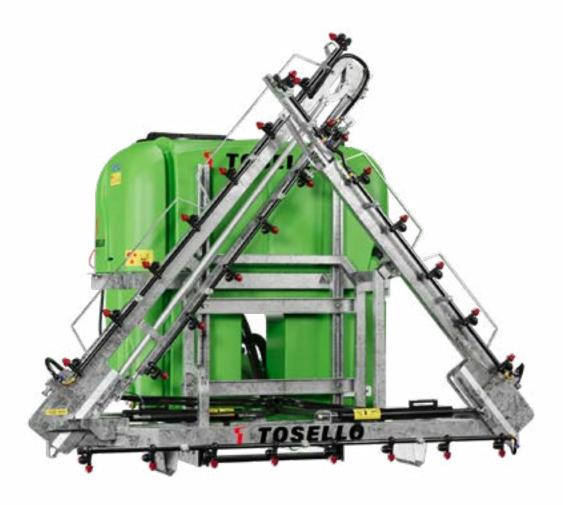
Linkage sprayer designed to cater to the requirements of greenhouse vegetable growers. Its distinguishing feature is the asymmetrical weed spray boom, which allows herbicides to be applied while working around the raised row layout typically associated with greenhouses. It comes in one size with a coverage of 7.5 m, and 25cm or 50cm nozzle spacing.
