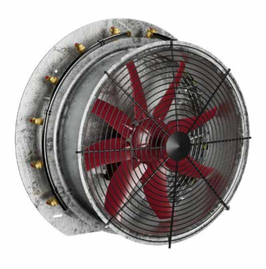
Rear-intake fan assembly with diameters ranging from 500 mm to 800 mm, glass-filled nylon 8-blade fans. The whole fan assembly is hot-dip galvanized to withstand even the harshest herbicides. The gearbox can be single speed + neutral or 2-speed + neutral.
