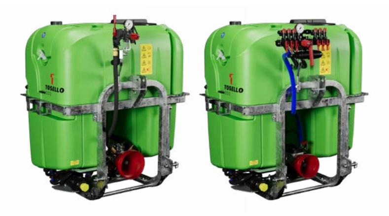
Boomless spray units with no fan assembly, featuring low-, medium- or high-pressure pumps depending on their intended use. They can be fitted with a wide range of accessories: lance for treating tall-trunked trees, T-boom for spraying trellis systems, weed control lance, inter-row booms, and chemical sucker remover.
