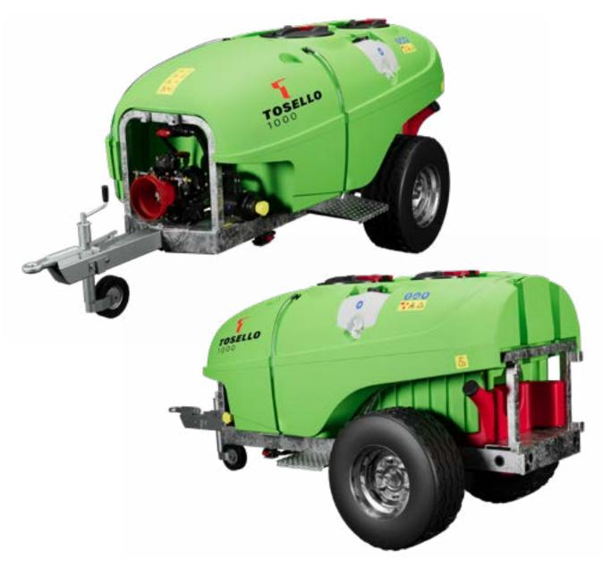
Boomless trailed spray units with no fan assembly, featuring low-, medium- or high-pressure pumps depending on their intended use. Capacity can be chosen in a range from 600 litres to 2000 litres. They can be fitted with a wide range of accessories: lance for treating tall-trunked trees, T-boom for spraying trellis systems, weed control lance, inter-row booms, and chemical sucker remover; or they can be used for watering plants on municipal garden beds, along roadsides, and hard-to-reach areas.
