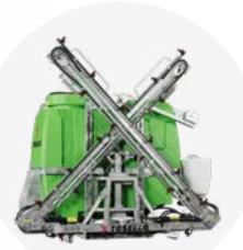
Model specially designed to cater to the requirements of medium-large farms, and contractors. It features P2-series booms with self-levelling and mechanical auto lock, or with tilt correction cylinder.
