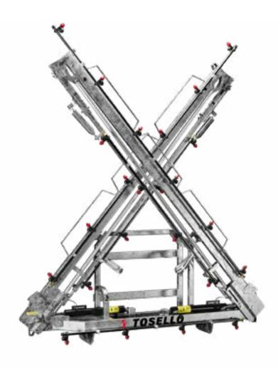
The L2 model, which has been tried and tested over the years and features a high level of reliability, is our entry-level hydraulic boom. Opening and closing is achieved, on each side, by a hydraulic cylinder and a tie rod: there is a clear benefit to this system, requiring just two double-acting hydraulic couplers to operate the unit. A question of practicality.
