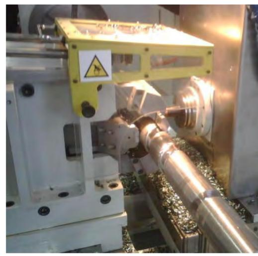
Our threader machines can be equipped by: end mills milling heads (our slanted bed models PLUS 400 and PLUS C and our models with horizontal bed F85 and F50); disc cutters milling heads (PLUS CD and PLUS C); whirling heads (our GRM models)
