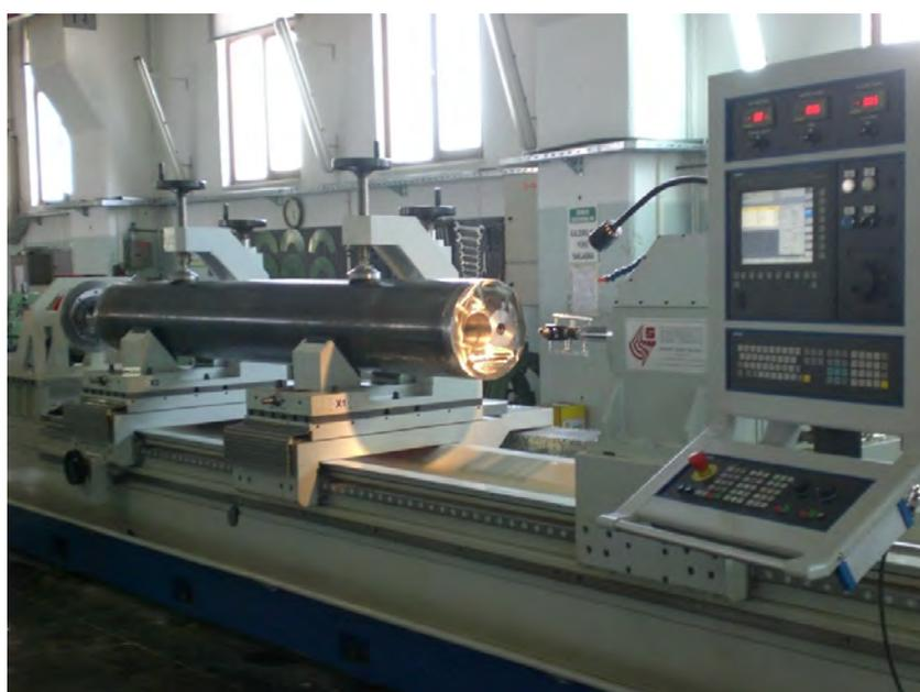
The model "SAPORITI PR" has a rotating workpiece with the option of having a controlled axis for internal profiling (**bottle boring**).
