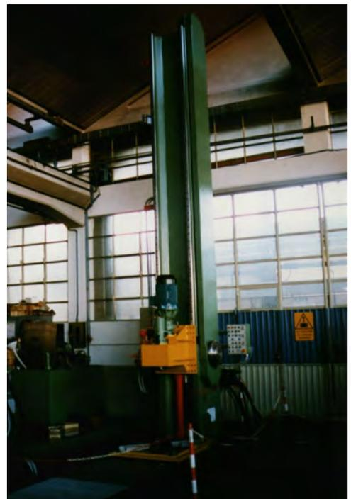
Also in production vertical lapping machines up to 5 meters.
