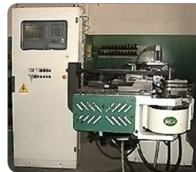
BLM NC863 CNC Tube bending machine 60 mm maximum tube diameter
