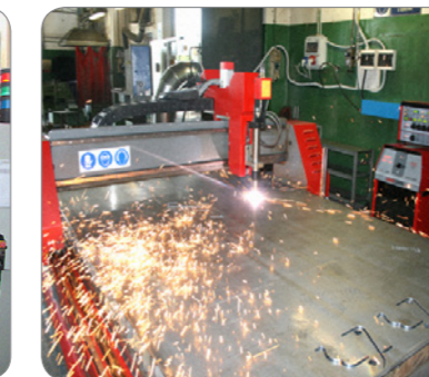
Plasma cutting machine For 3000 x 1500 mm sheet metal max width 25 mm on iron
