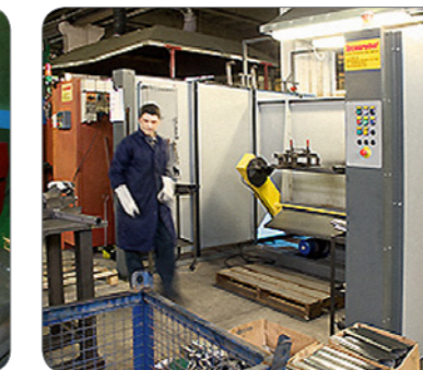
Fanuc Arcmate 100 I welding robot Rotating benchtop positioner with dual lathe and controlled axes
