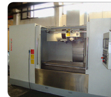
Microcut 1600F Work centre travels 1600 x 800 x 800 mm
