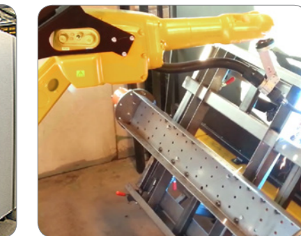
Fanuc Arcmate 100 I welding robot Rotating benchtop positioner with dual lathe and controlled axes
