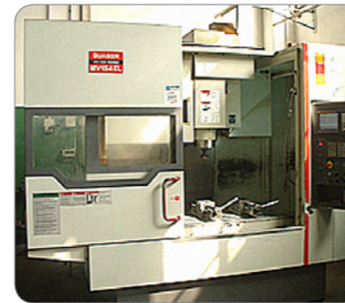
Quaser MV154EL vertical machine centre (travels 1030 x 500 x 500)
