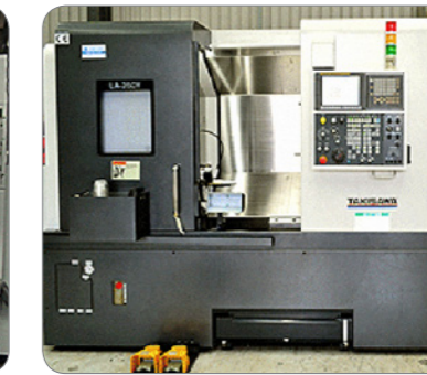
TAKISAWA LA 250 Lathe 350 mm max turning diameter. 635 mm max turning length.
