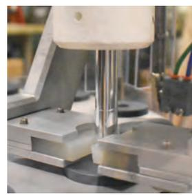
*Filling and capping monoblock for mascara, semi-automatic solution equipped with pneumatic rotary table, with adjustable rotation speed. Through the step movement, the containers enter the dosing station where 1 syringe for semi-dense liquid products doses the product. The cap is positioned manually and in the capping station is closed with a special screwing unit with a control unit for adjusting the tightening torque. PRODUCTIVITY: 1.000 pcs./h.*
