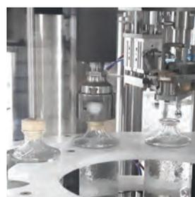
*Automatic rinsing, filling and capping monoblock for whiskey and gin bottles. Plant placed on adjustable feet, each part in contact with the product is in AISI 316 steel, and is built according to CE standards.*
