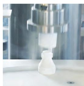
*Mixing, filling and capping line for talcum and cosmetic powders, in bottles of 210 g. The system consists of a mixer and a liquid pump capable of dosing fragrances and then create the compound that is then transferred to a 5-nozzles filling machine for dosing talcum powder into containers. The loading of the cap is automatic and the capping monoblock with a pressure closure head completes the packaging.*
