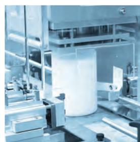
*Filling, sealing and capping line for the packaging of cosmetic creams in 250 and 500gr jars.*
