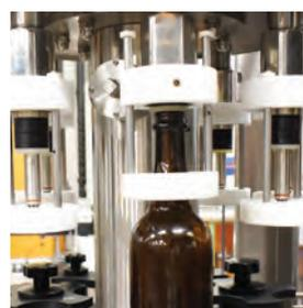
*Automatic filling and capping monoblock for cylindrical glass bottles of 75 and 50 ml of non-foaming beer.*
