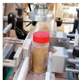
*Automatic filling, freshness sealing, capping and labelling line for powders and granules, in jars from 20 to 500gr. The solution is equipped with: loading table; loading hopper complete with level sensor; doser with 4 vibrating channels equipped with weight control system and telescopic funnel adapters; automatic feeder of caps with system pick & place; capping machine for screw caps; induction system for sealing under-cap; labeller M3010 for wraparound and front/back application.*
