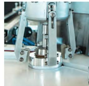
*Filling and capping monoblock for cosmetic creams and serums. Packaging solution for 3 different containers, screw caps and dropper caps.*
