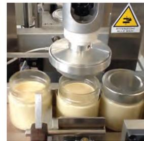
*Filling, capping and labelling line for spreadable cream in jars from 20 to 680 ml.*
