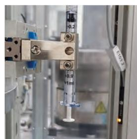
*Filling and capping monoblock, state-of-the-art solution for 4cc and 8cc syringes.*
