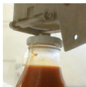
*Filling and capping line for jars from 50 to 1000 ml. The machine has a loading and unloading plate and a feeding belt with centering system, to stop the product in the dosing area. The filling station has 2 volumetric nozzles and is complete with heated cavity hopper, agitator and level sensor (sonda). The capping station is with automatic feeding for twist off cap, capping head and steam injection area to prevent the deterioration of food. PRODUCTIVITY: 1.000 pcs./h.*
