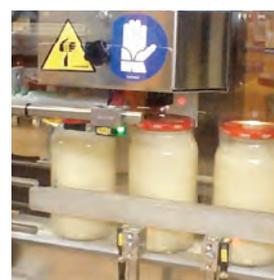
*Filling, capping, sealing and labelling line for jars of 200 and 500 gr. The line is composed of: a rinsing machine; a filling station with 4 nozzles and hopper with level sensor; a capping station with automatic feeding for twist off cap; a sleeve station equipped with shrink tunnel; and finally a labelling line M3010 for front back and wraparound application of the label on the jar. The control and monitoring of the machines is via PLC with easy and intuitive touch-screen system.*
