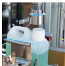
*Automatic filling and capping line for tanks and cans with capacities from 250 to 1000 ml. The plant is equipped with: 1 filling station with 4 volumetric dosers with brushless motor and antifoam system; product transfer pipes with non-return valve; 1 TTB capping station with one head for screw caps and format changeover for pressure caps; outfeed rotary table; conveyor belt to convey containers to filling and capping stations.*
