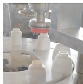
*The new Monoblock PMR MFC 22 is the suitable solution for filling liquid, semi-dense and dense products in plastic and/or glass containers, with screw cap or twist-off.*
