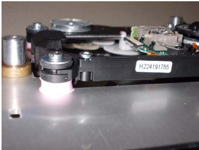
New rubber pink feet isolating mechanism from alluminium plate
