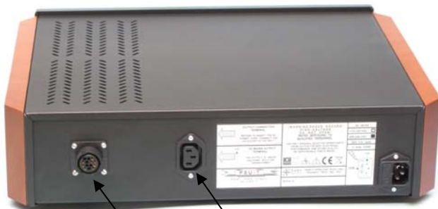
Output ac power for audio components as preamp/power
