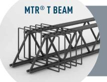
has to be shuttered and propped during the assembly and casting phase of the floor. It does not have the bottom plate and it is completely embedded in the cast-in place-concrete.
