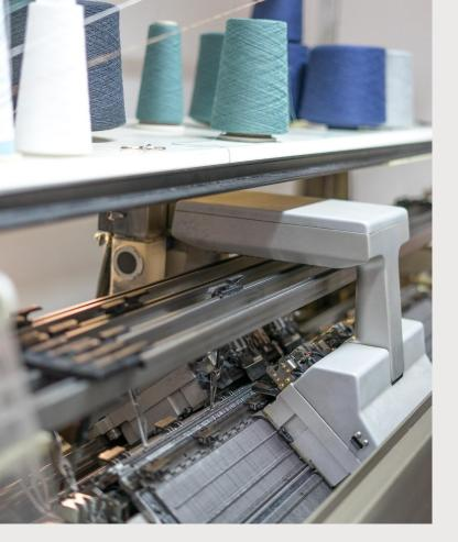
Here in Tasselli we can offer our clients 7, 12, 16 and 18 GG machinery. We work both with hand operated and Shima Seiki electronic machines and we are able to produce any kind of fully-fashioned knit from inlays to jacquard patterns using the finest natural yarns with every type of contouring.
