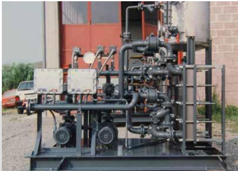
Cooling skid built for the company Nuovo Pignone in Florence at the end of 80 years.
