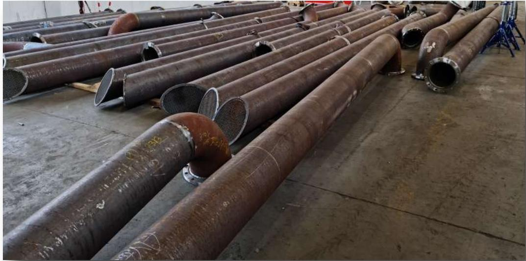
Carbon steel prefabricated piping
