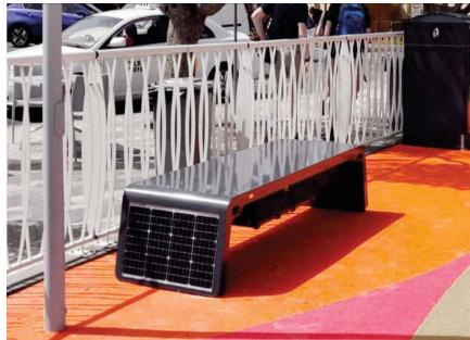
The Smart Denver bench combines technology and sustainability in a clean design suitable for any application. It is made of galvanised and powder coated steel and it is endowed with two photovoltaic panels on the side and a battery for energy storage in the opening compartment under the seat. The battery can power 4 USB doors that are located to the corners of bench, as well as the LED lights provided for dark hours.
