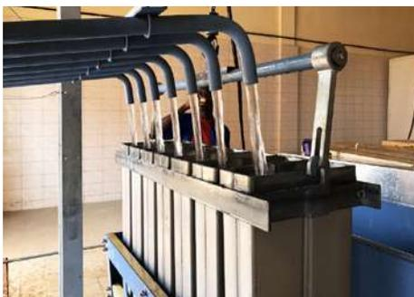
Filling phase of the moulds with water
