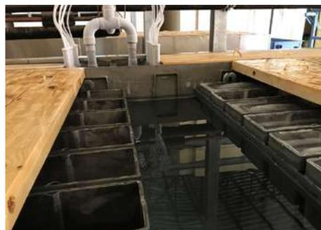
Stainless steel moulds immersed in brine
