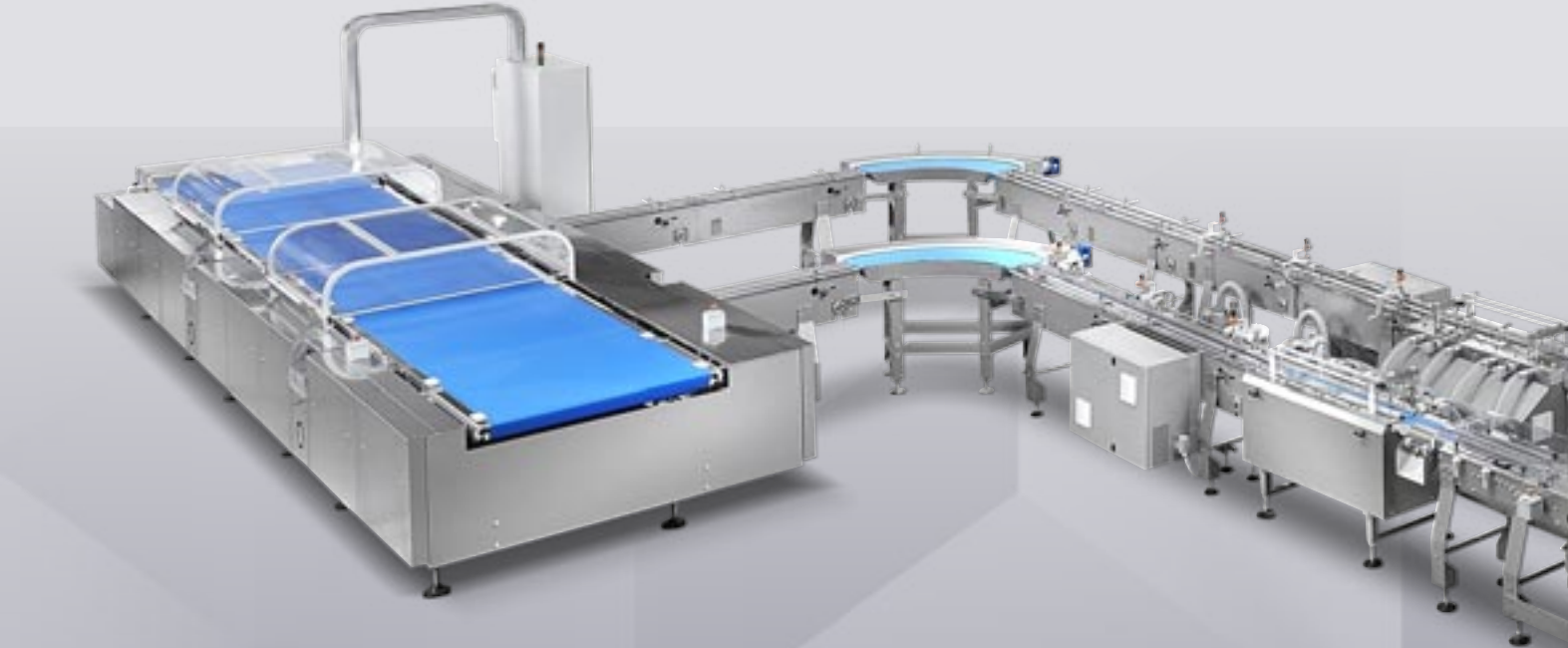
Row distribution system combined with electronic numerical loader for biscuits on edge
