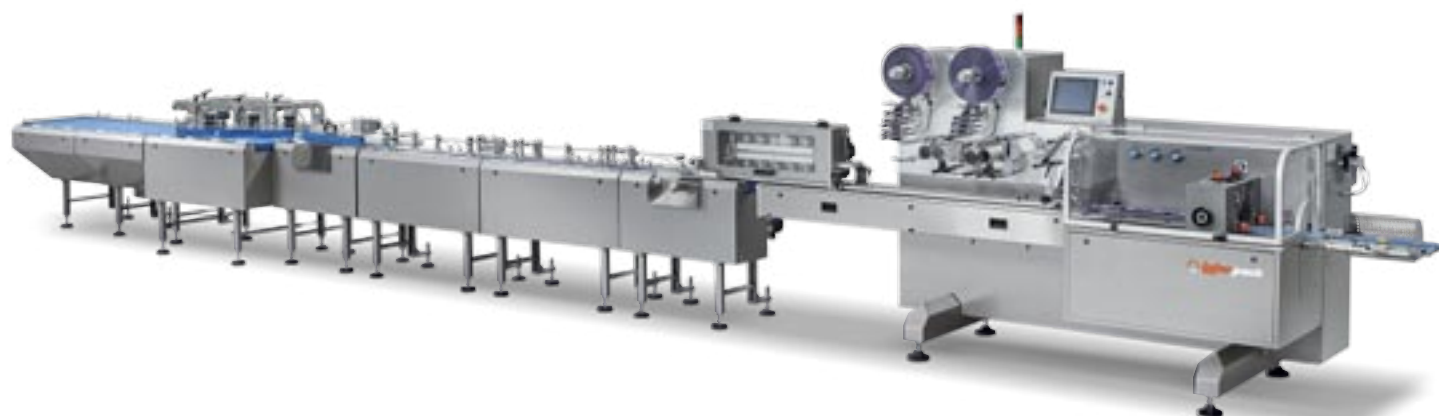
In-line feeding system with streamers suitable for small products arriving randomly
