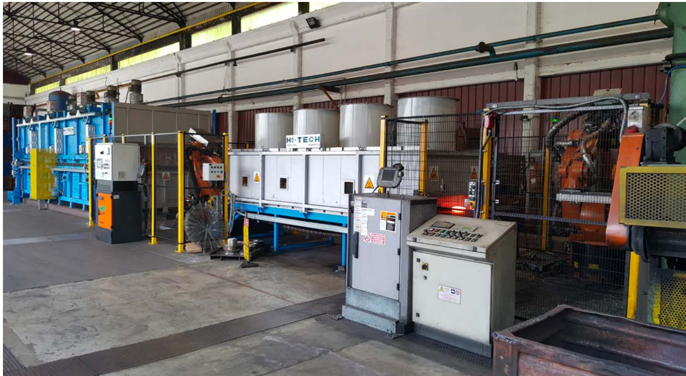
Belt type continuous line for isothermal annealing after forging.
