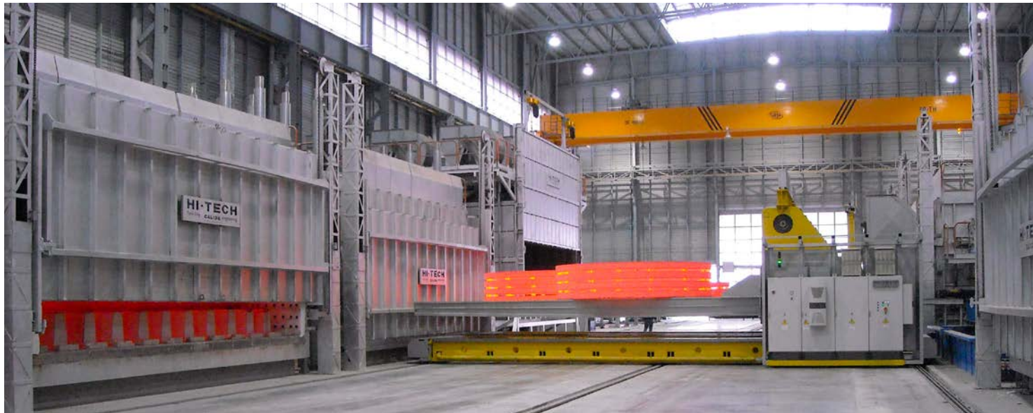
Heat treatment of large size forged rings (batch type line for 8 meters diam. rings).
