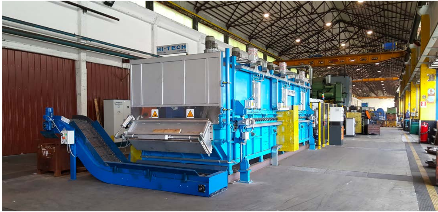
Belt type furnace for isothermal annealing.
