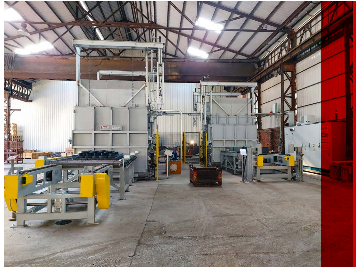
Continuous lines with roller type for automotive parts.
