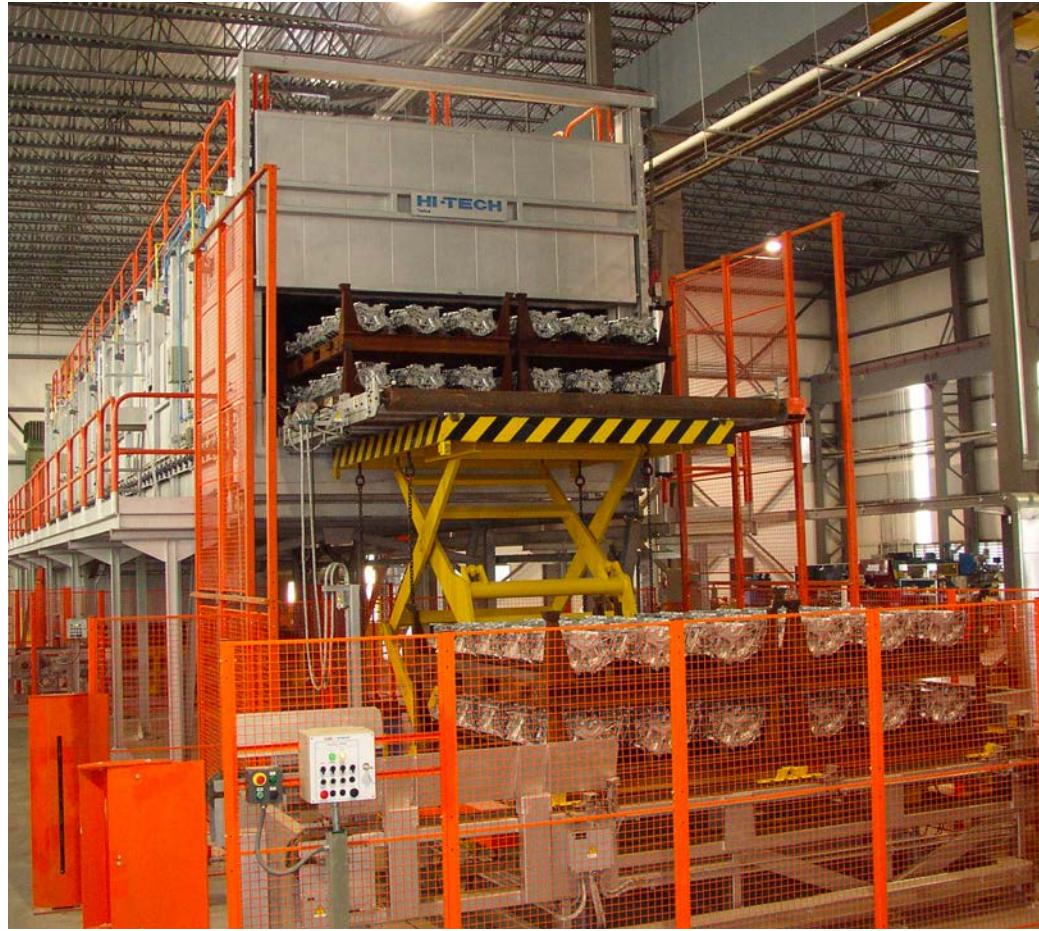
T5 heat treatment for aluminium engine blocks V6.
