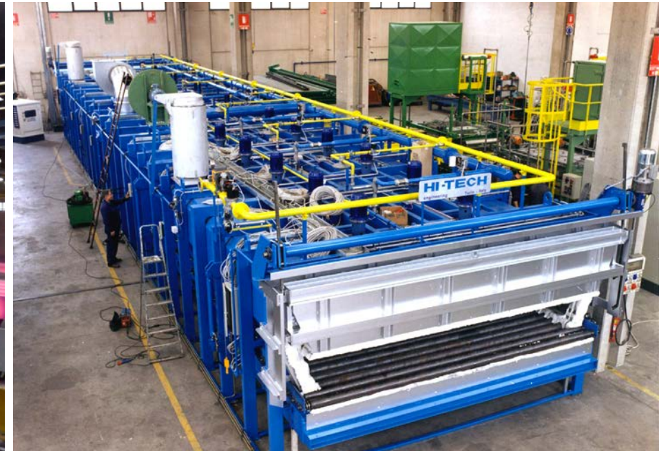
Continuous lines with roller type furnaces.
