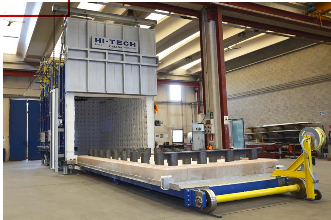
Car bottom furnace for the heat treatment of different parts, globular annealing and isothermal annealing.
