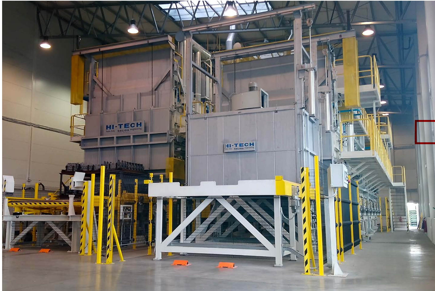
Heat treatment line for different cylinder heads, with air quench and water quench.
