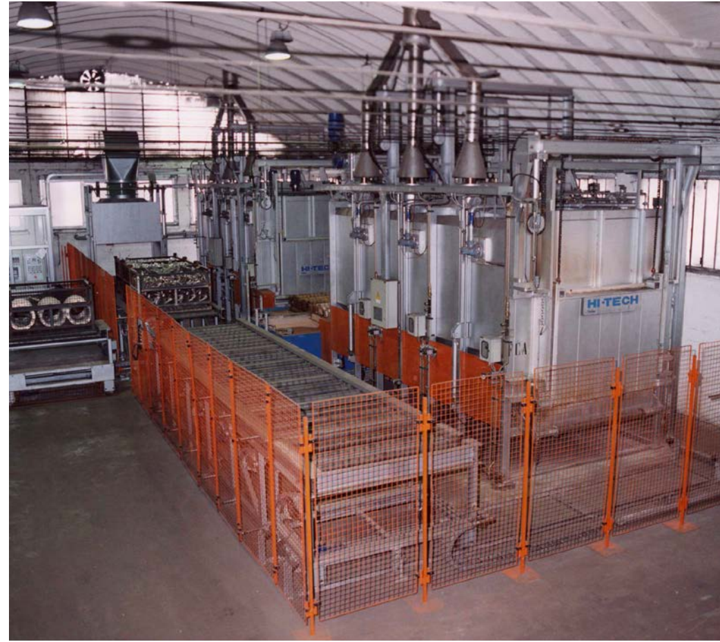
Heat treatment of aluminium parts for the automotive industry.
