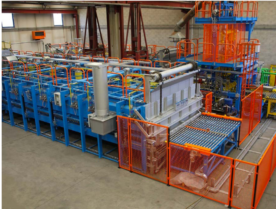
Continuous line for quenching for Oil & Gas parts.
