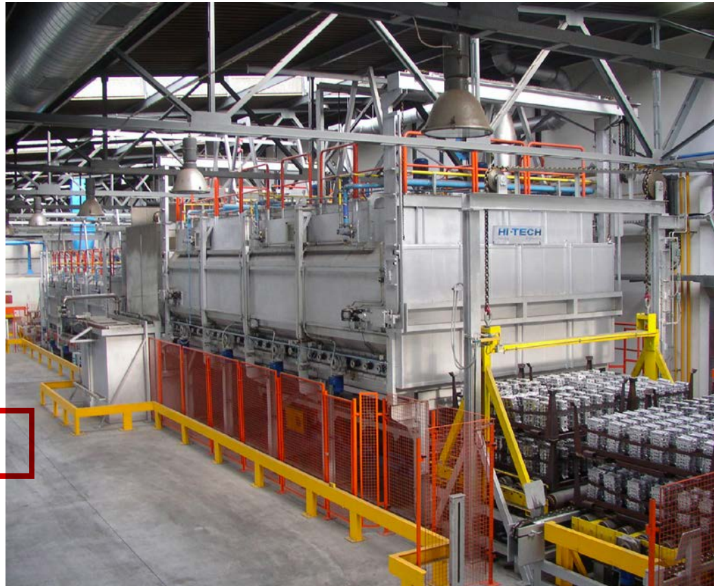
T6 heat treatment and thermal sand removal for aluminium engine heads.
