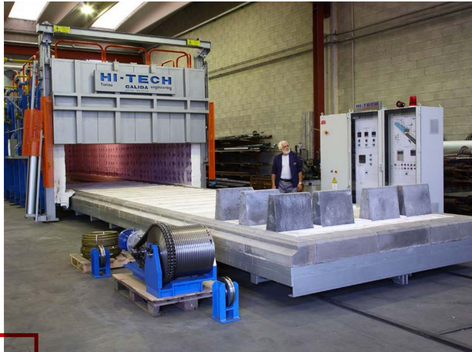
Globular annealing heat treatment of rings for bearings.
