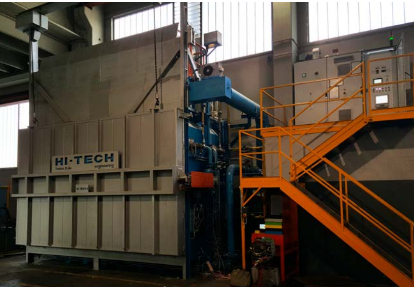
Batch furnace for aerospace parts.
