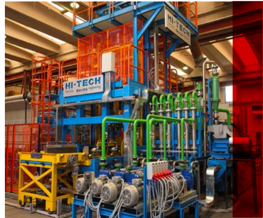
System for individual forced quenching of tool joints.
