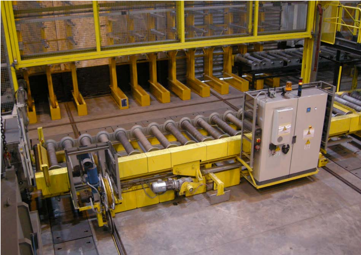
Shuttles and transfer roller tables.
