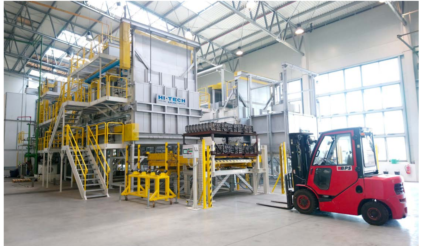
Heat treatment line for automotive parts with air quench and water quench.
