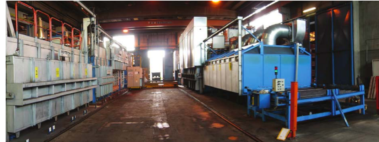
Batch type lines with box type furnaces and charging machine.
