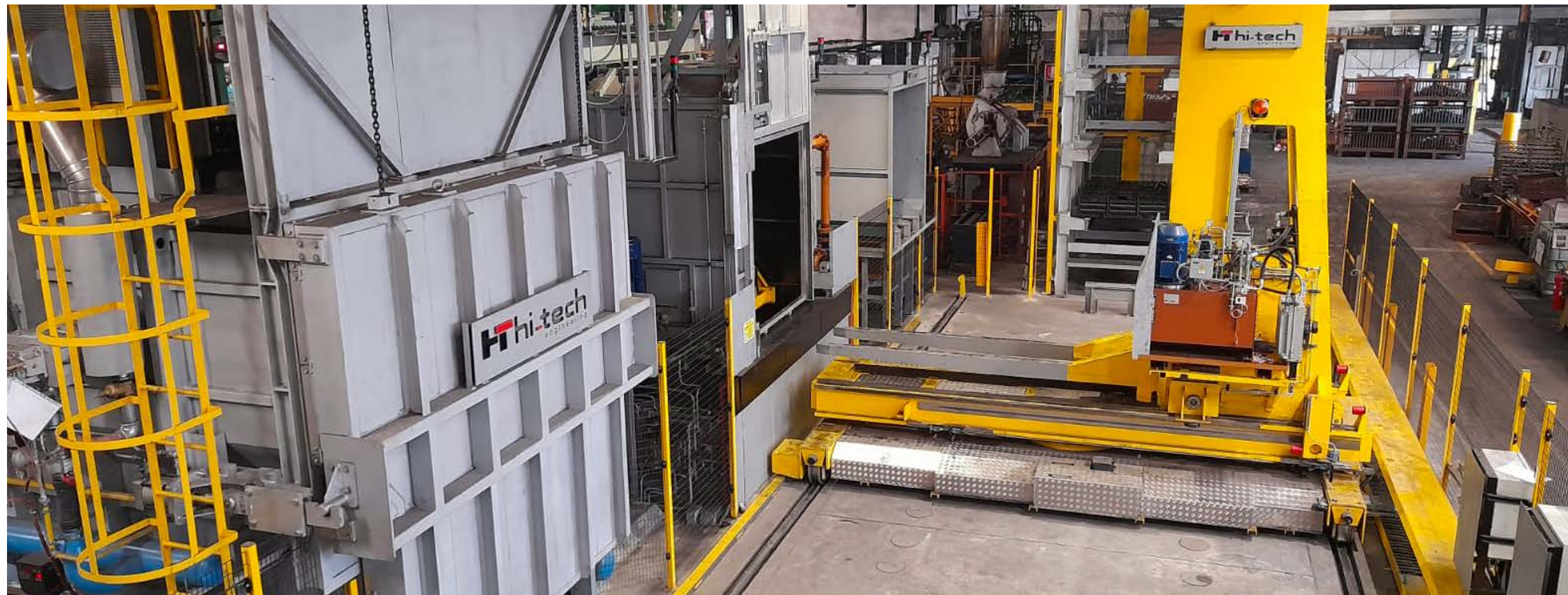
Versatile line with oil quench for automotive parts, agricultural and undercarriage products.
