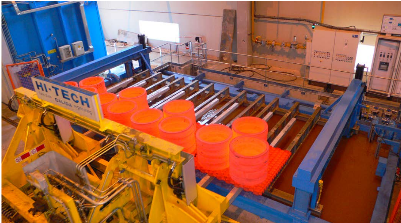
Water-Polymer quench of rings and wheels.
