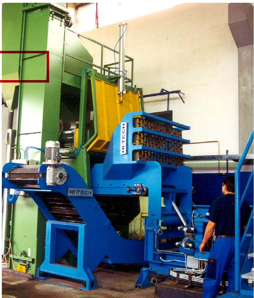
Tilting device for continuous roller type furnace.
