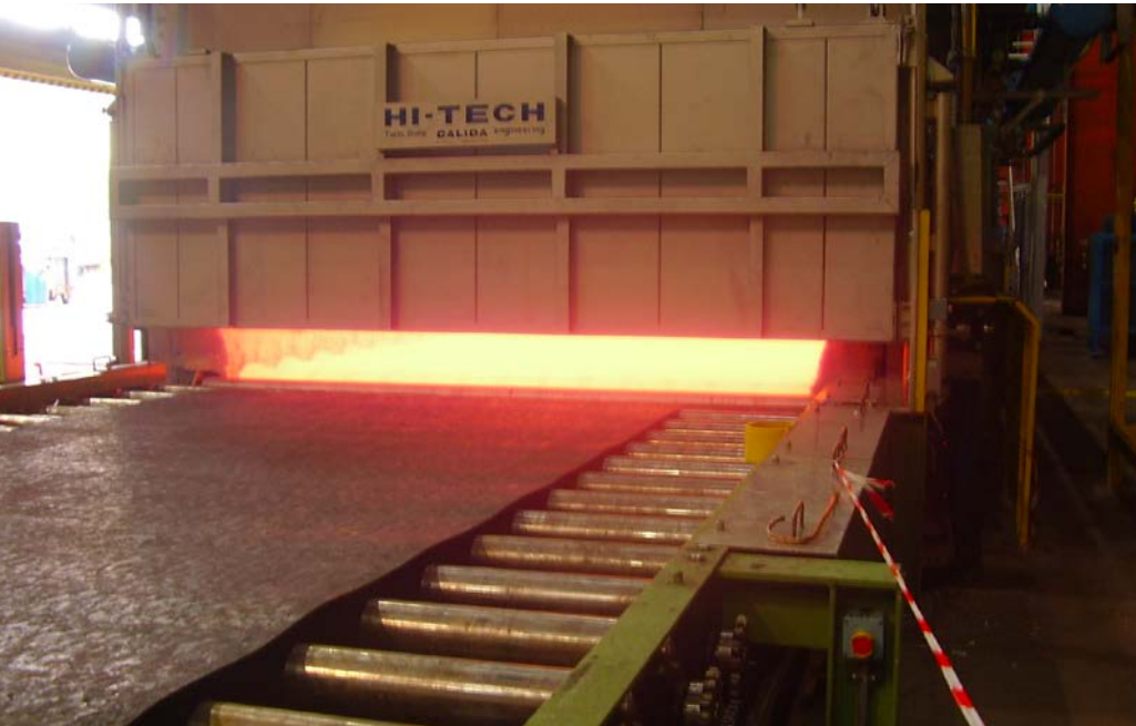
Continuous lines with roller type furnaces for plates.
