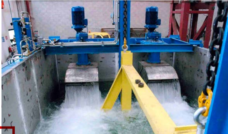
Direct quench after forging, parts for undercarriage.
