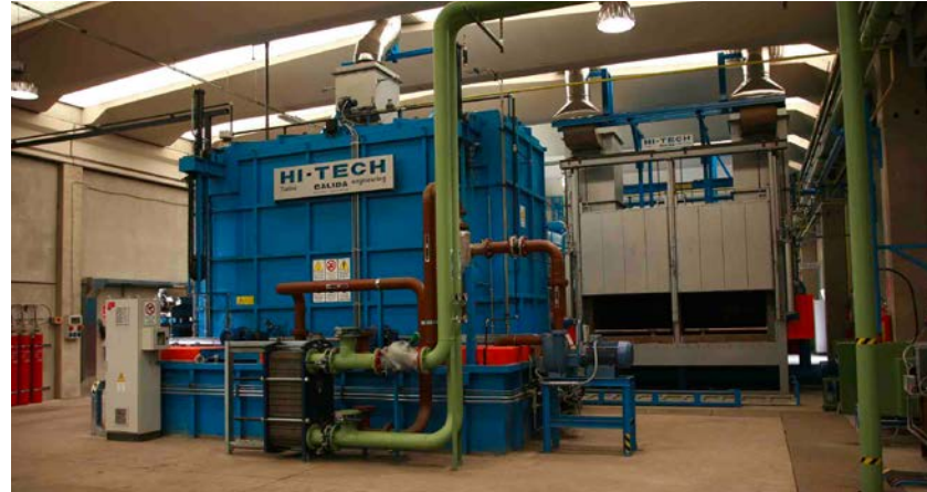
Water quench installation for Oil & Gas parts.
