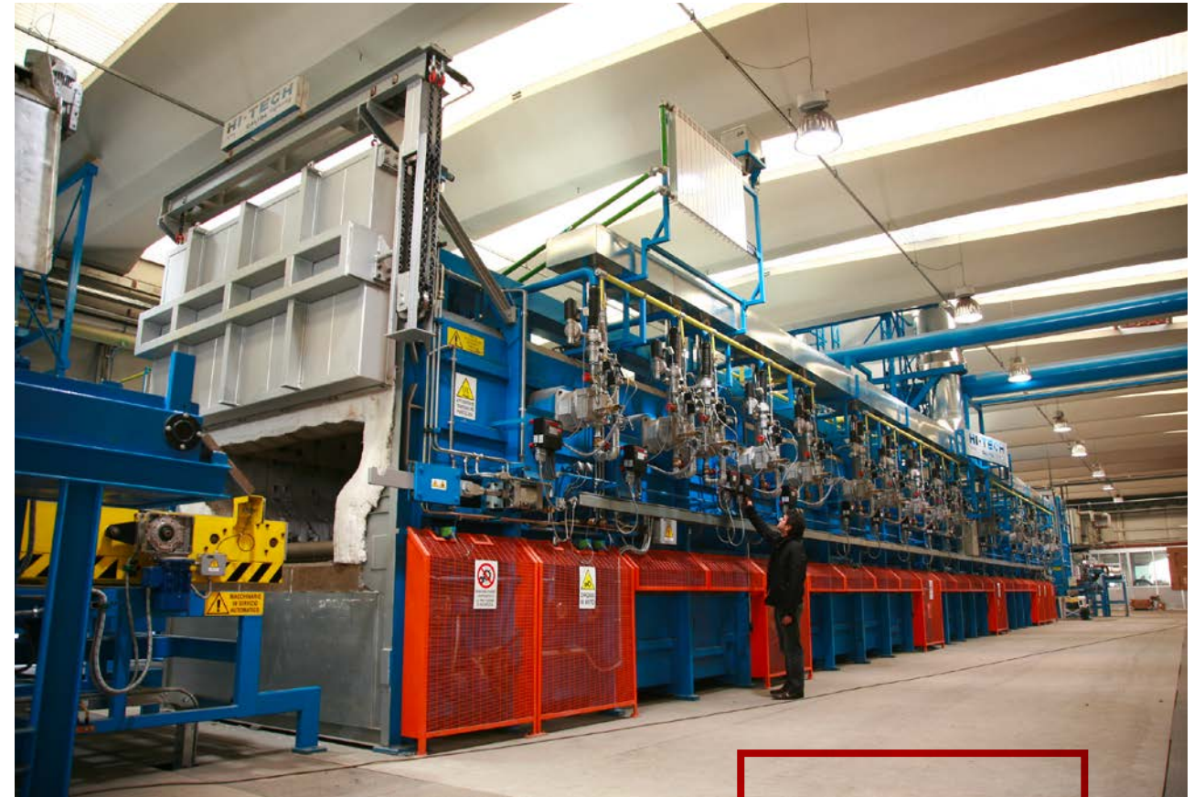
Tunnel type line for heat treatment of different parts inside baskets.
