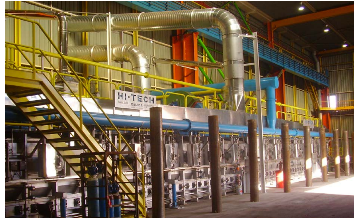
Continuous lines with roller type furnaces.
