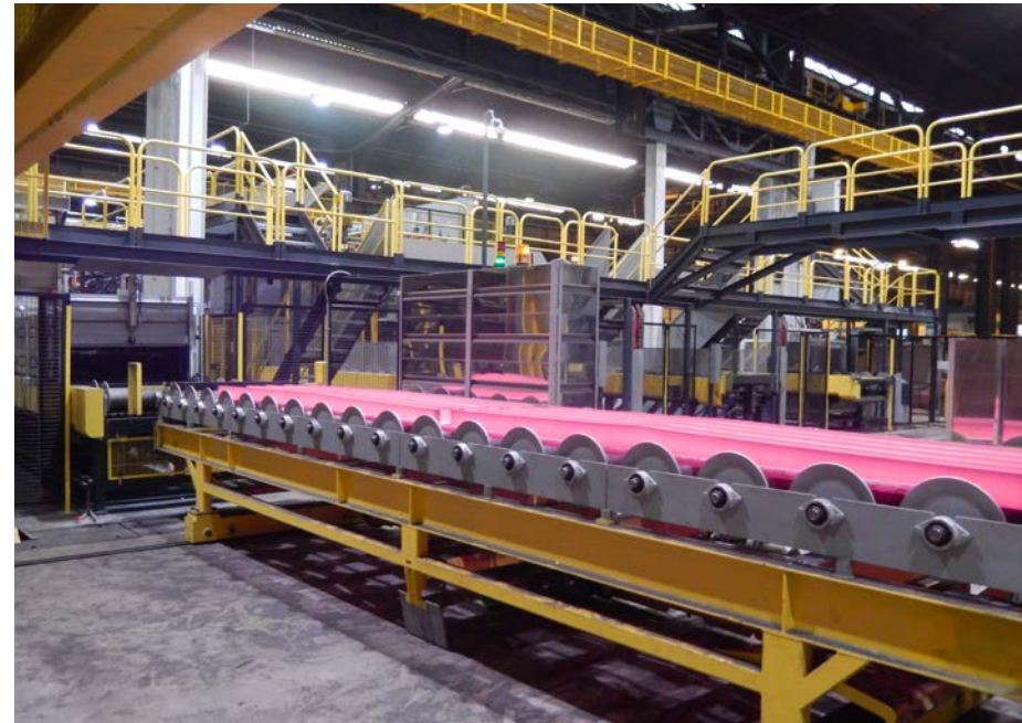
Continuous lines with roller type furnaces for up to 7.5 meters bars.
