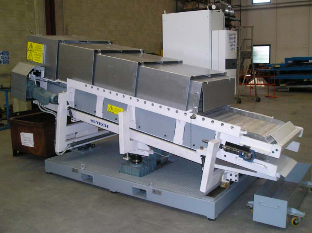
Conveyor for cooling of connecting rods.
