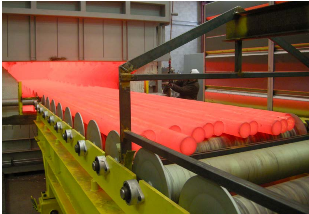
Tunnel type installation for bars.
