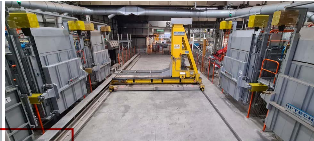
Heat treatment for engine blocks and cylinder heads.
