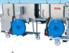
LAV10 DMATIC TRAY WASHER WITH CHEMICAL TREATMENT TUNI UP TO 600 CONTAINERS/HOUR
