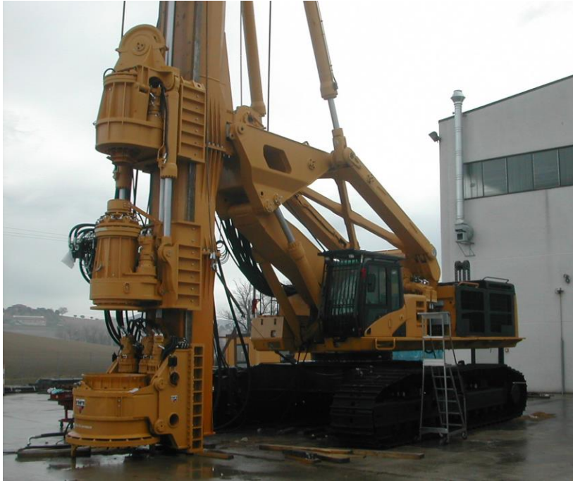
AF460 IN MULTIROTARY VERSION (SOIL-MIXING TECHNOLOGY FOR ANTI-SEISMIC PILES)
