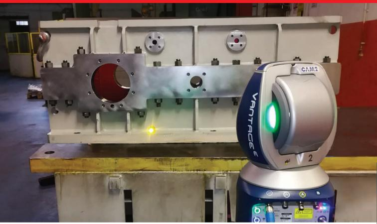
Averoldi can also boast a dimensional testing department, that not only provides certification on the parts internally manufactured but can offer the service to third parties too; releasing a type A1 certification.
