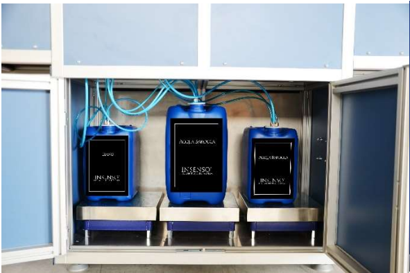
3-Accommodation provided for 3 tanks of 10 or 20 liters with recognition RFID
