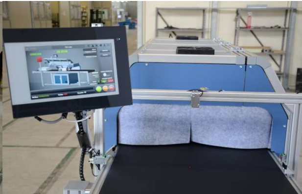
2-Tunnel entrance, with control console, for digital setting of disinfection
