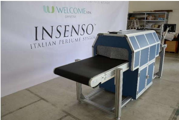
1-Exit from the tunnel with the function of the conveyor belt in line or go-back, depending on the number of operators
