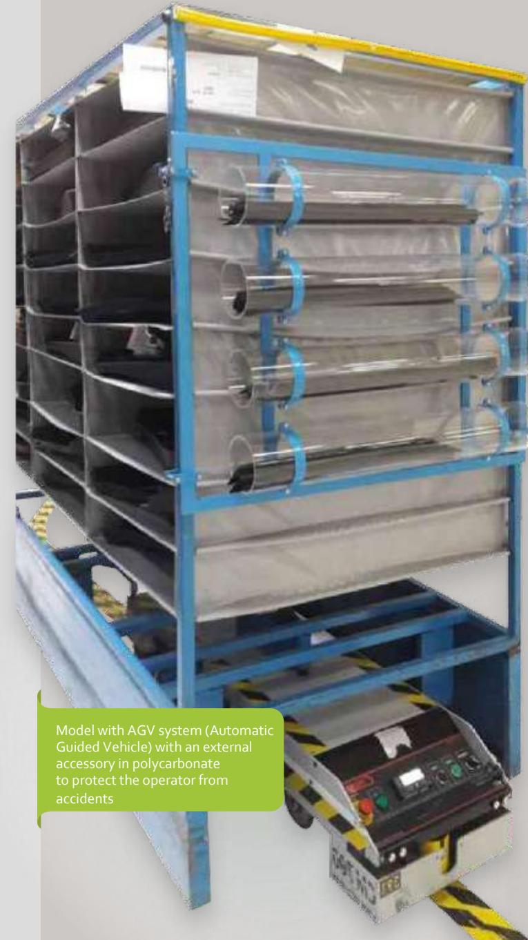
Model with AGV system (Automatic Guided Vehicle) with an external accessory in polycarbonate to protect the operator from accidents
