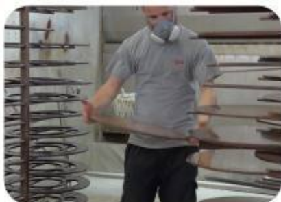
Drying after spray painting
