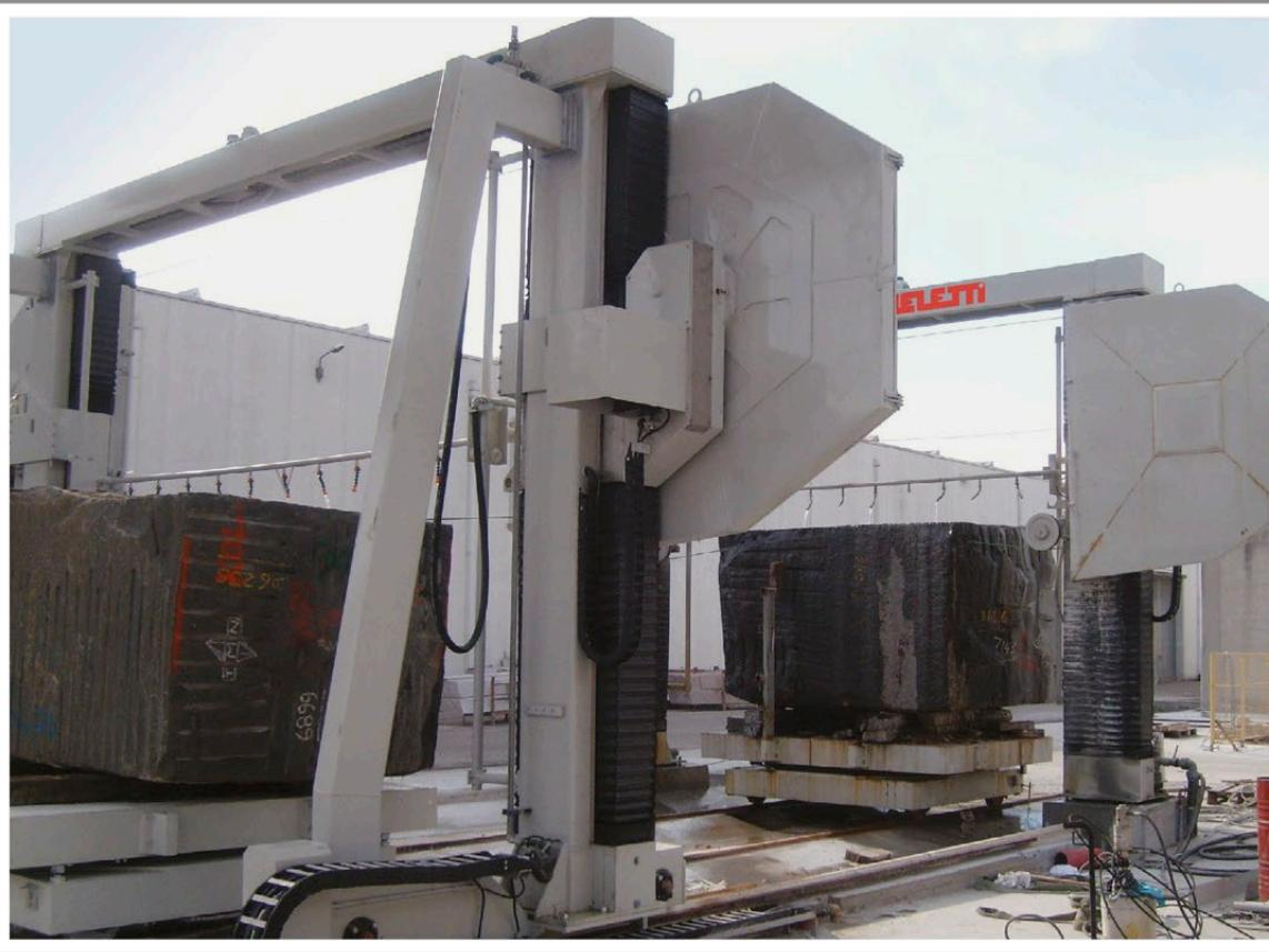
The diamond wire plant DIAMSTAR TECH, manufactured in 3 versions, stationary, mobile on rails and double (stationary + mobile), has been conceived for block squaring and thick-slabs cutting of marble and stones and, in the model with variable rim speed also granite.
