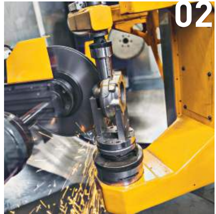
02 Deburring spindle with diamond wheel
