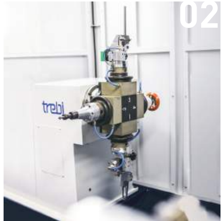
02 Turret revolver unit for pneumatic tools
