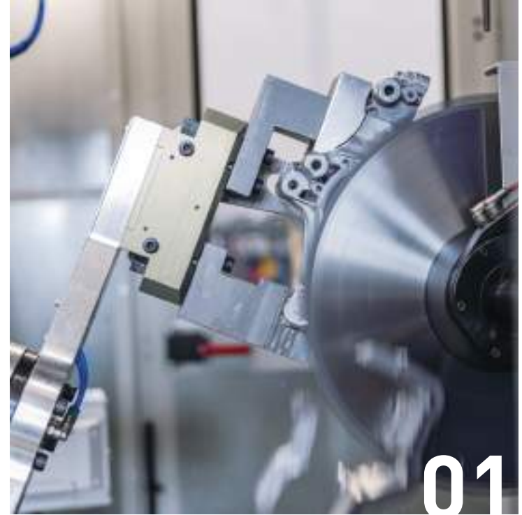
01 Detail of the cut pouring branch
