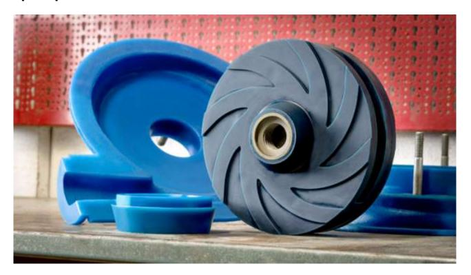
Hot cast polyurethane spare parts represent a worthy alternative compared to new and expensive original ones made of rubber or other plastic materials for industrial machinery, thus allowing a relevant saving on upkeep costs.
