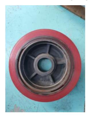
Forklift truck wheels can be made of many materials, each one with different characteristics, in terms of durability, resistance to tearing, cutting, water and chemical action but most of all to high load.
