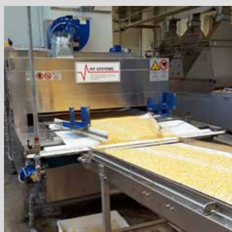
➤ Sanitization of corn 1000 Kg/h throughput
