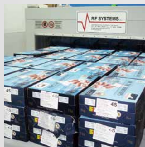
➤ Defrosting of packaged shrimps 1500 Kg/h throughput
