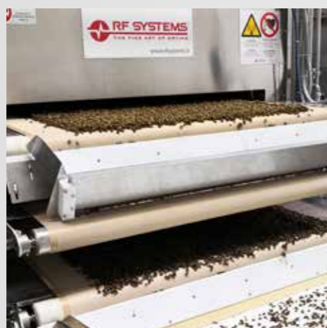
> Drying of candied fruit citrus 1000 Kg/h throughput
