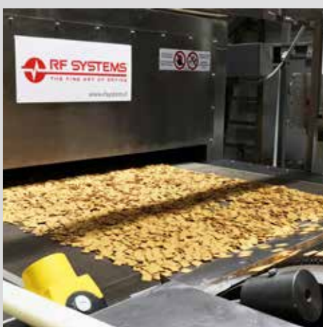
> Drying of crackers 600 Kg/h throughput
