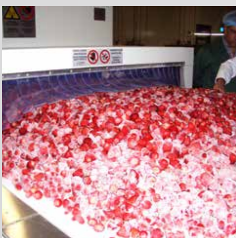
➤ Defrosting of IQF strawberries 1000 Kg/h throughput
