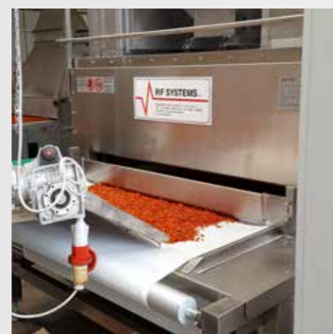
➤ Pasteurization of dried tomatoes 800 Kg/h throughput
