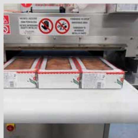
➤ Pasteurization of packaged croissants 300 Kg/h throughput
