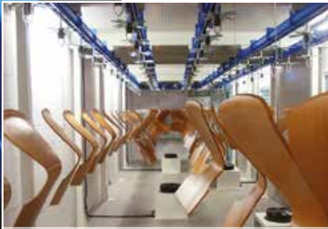
In the monorail conveyors, the function of bi-planar chain is twofold: traction and load-bearing.
