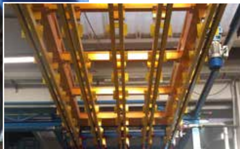
The use of a manual conveyor is a logical and valid choice where handling does not require excessive rhythm or overly complex production cycles.
