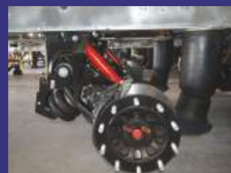
9 ton SAF axles, liftable-fixed-steering
