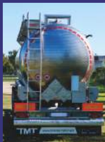
The tank body is made of AISI 316 stainless steel, internally polished
