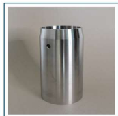
F46754-1000 PROTECTOR AXLE, MLG A318 - A319 - A320 - A321 (depending on MSN, otherwise the applicable p/n is Q47316, different from F46754-1000)
