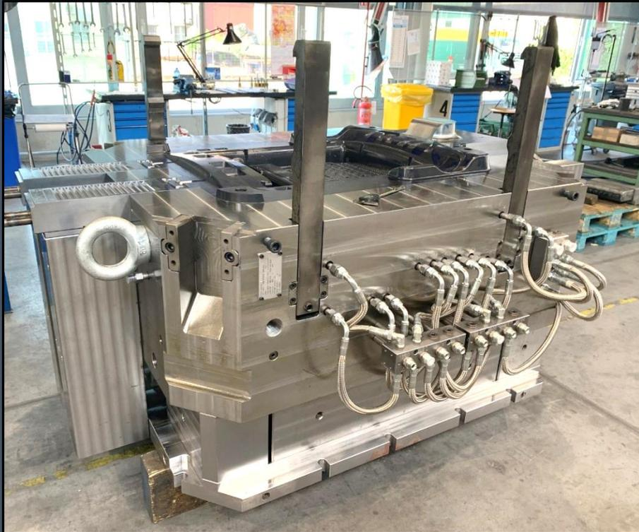
Tool - Inverter/Battery housing
