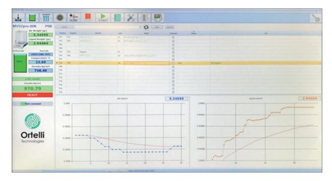
Fully automated sequence reading, including control tests and correct detection of measured parameters.
