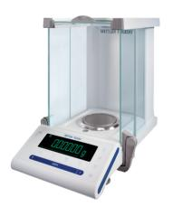
Analytical Electronic Balance with underplane support weight to position the support sample in the measurement area of the **MVS2pro**. The balance suggested is at 5 decimal places in grams like: MS, XSR, XPR Series. (d= 0,01 mg)
