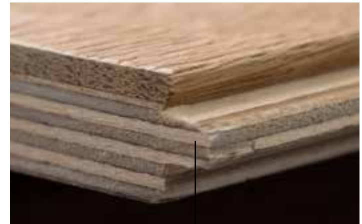
Tongue with profile to ease the connection
