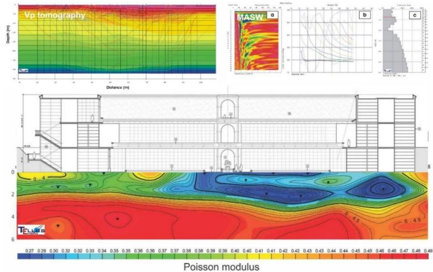
*Stratigraphy reconstruction by refraction seismics*
