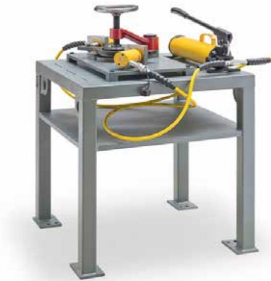
ROLL BEARING PRE-LOADING DEVICE
