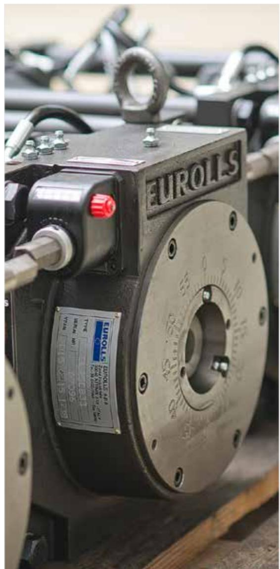
CA and CB cassette models are mostly used to process low carbon wire for the construction industry. These cassettes are normally mounted on one or more drafts machines, where wire is reduced and/or deformed, used as a base for lattice girders, mesh, or generally reinforced concrete application.
