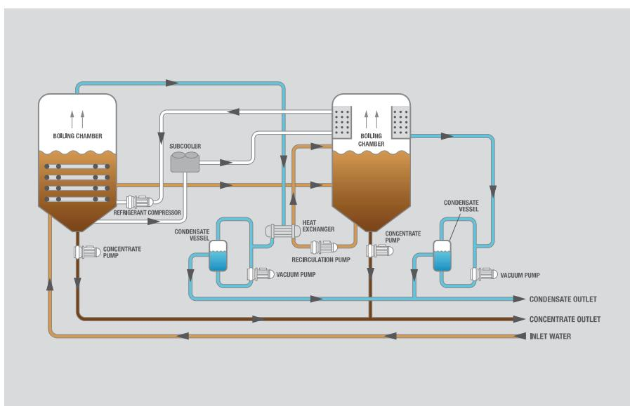
WITH SCRAPER FOR ENCRUSTING LIQUIDS. DISTILLATION THROUGHPUT 20 to 125 l/h
