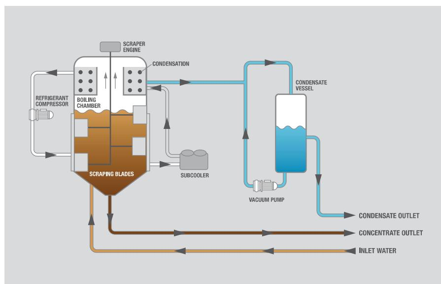
WITH SADDLE JACKETED HEAT EXCHANGER. DISTILLATION THROUGHPUT 10 to 42 l/h
