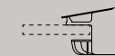
External top access Top access esterno L 40 cm, W 23 cm, H 17 cm L 15 ¾", W 9", H 6 ¾"
