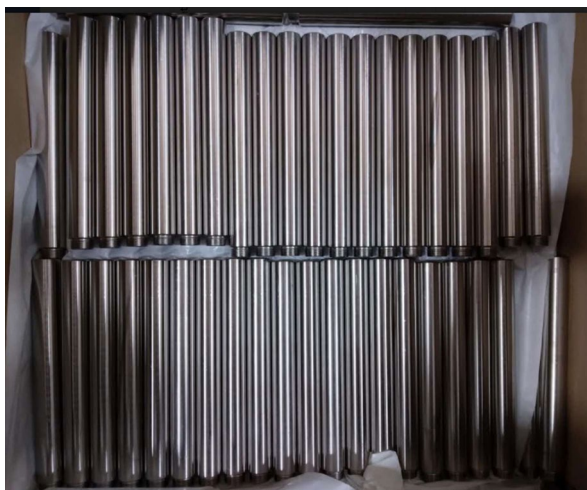
Pins back from 20 \mu m nickel plating treatment
