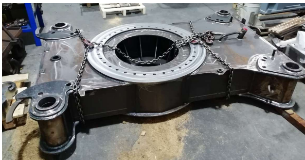
Base frame bearings flange after machining - aerial platforms application
