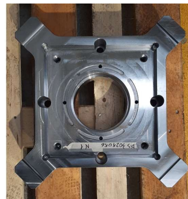
Mold holder - hot forging presses application
