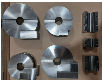
Bending matrices – pipe bending machines application
