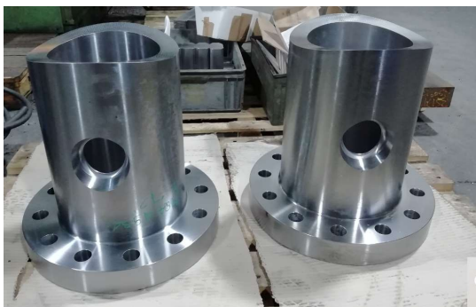
Nozzles – oil&gas offshore application
