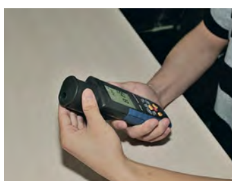
Rotating selector for Alpha "A", Beta "β", Gamma "γ" and "X-ray" radiation detection
