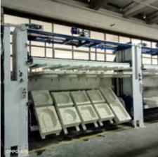
The machine consists of a metal structure that supports a mobile platform on which the lower half-mould is anchored, and an upper platform on which the upper half-mould is anchored and which has the function of keeping the mould closed.
