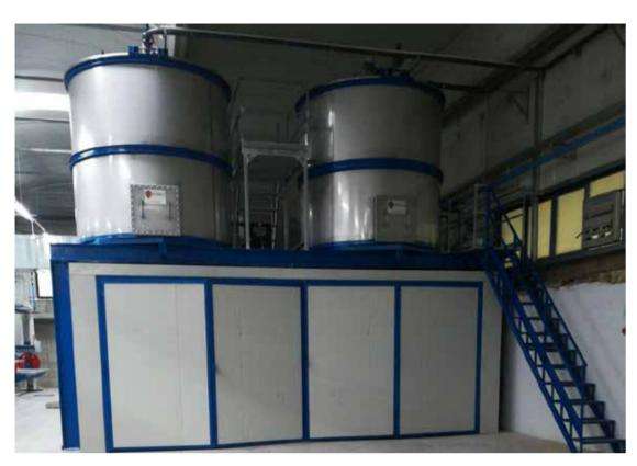
The sanitary ware dryer is designed for drying plaster molds of all types and sizes The dryer consists of:
