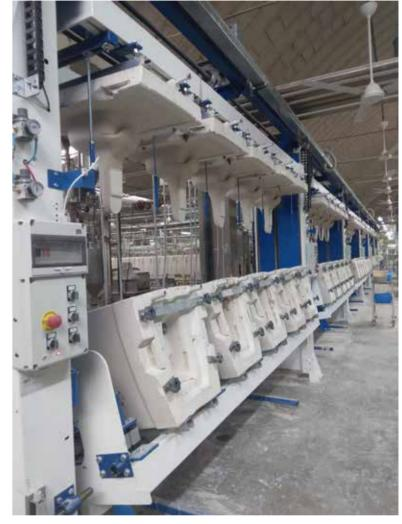
Low pressure casting benches, for all kinds of sanitary ware Each casting machine can accommodate up to 6 moulds, upon customer request.
