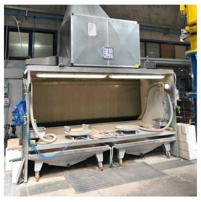
There are two removable lathes, two trays for dust collection and grid on the ground.
