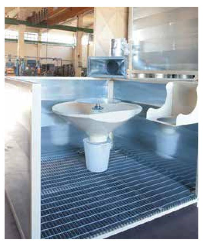
Cabin for manual sanitary finishing raw, equipped with hood and blast chiller for fine dust.
