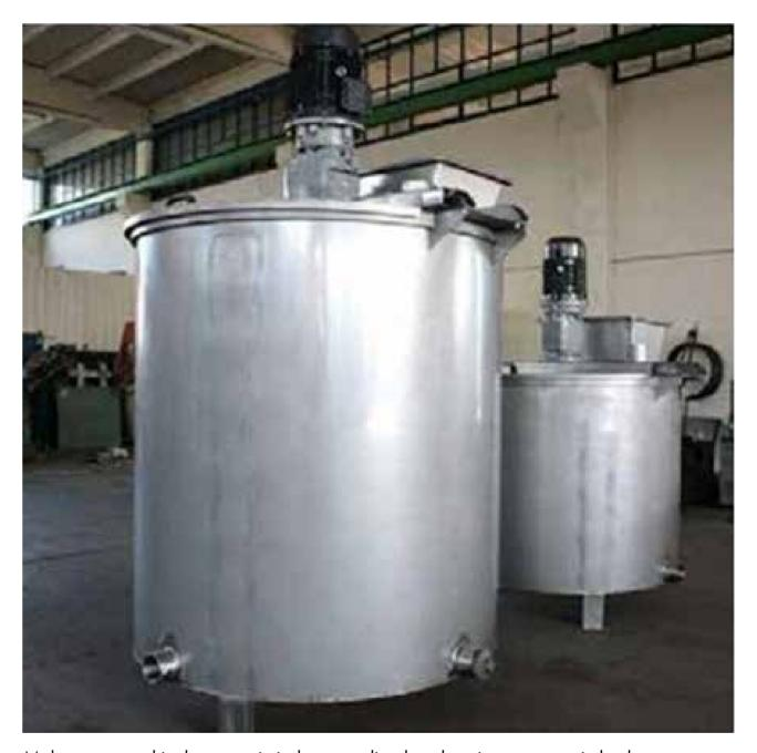
Melters are used in the ceramic industry to dissolve clays in water to mix barbs or enamels with other components and to avoid sedimentation of heavier components in suspension.
