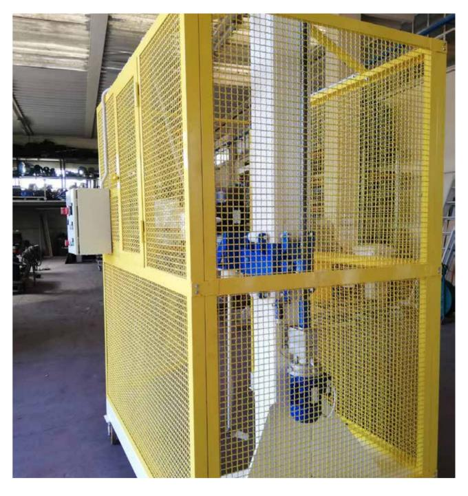
The wheeled stirrer is used for dissolving ceramic raw materials for the preparation of mixtures, glue solutions and mixing glazes
