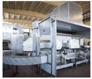
The booths are completed by a powder sucking system with fans. The productivity is from 2 up to 300 pieces in 8 hours, depending on the piece dimension. The plant is completed with feeding pumps, water recycling and electrical plant.
