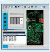
The VIVA software includes a graphical repair environment, which enables the user to locate and view the parts of the PCB which have failed during the test, facilitating repair operations.
