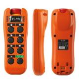
EVO is the ELCA handheld for lifting and handling applications with 6 double release buttons, a programmable aux, Start with electronic key, mushroom stop. 4 feedback signal LEDs. Internal Lithium battery, replaceable (40 hours of continuous use). Programmable auto-shutdown, IP65 degree of protection.
