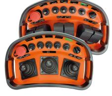
SFERA is similar to the PUNTO model, but is slightly larger to house 3 single or double axis on/off joysticks or 3 proportional or 6 single axis joysticks, 5 toggle switches, extractable activation key and Stop button.It can be customised to meet the specifications provided by the customer. Various actuators are available.
