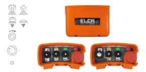
PIC is a compact waist portable radiocontrol created for forestry winches and a variety of industrial applications. 3 toggle switches to perform 5 commands (up to 8 with second function), mushroom stop button. Led "CHECK" indicates to the operator that the radio connection with the receiver is active.
