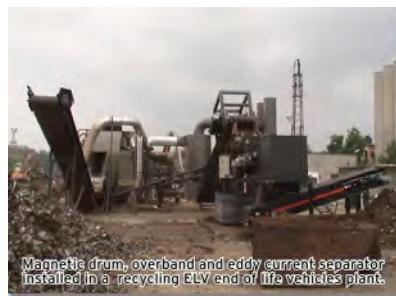
Magnetic drum, overband and eddy current separator installed in a recycling ETV end of life vehicles plant.
