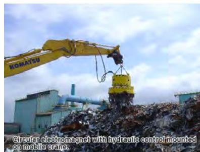
Circular electromagnet with hydraulic control mounted on mobile crane.
