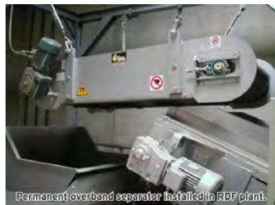
Permanent overband separator installed in RDF plant.
