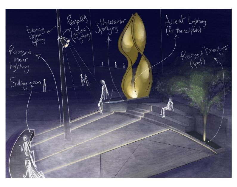
The first solution involves recessed linear lighting installed in the ground, radiating outward from the seating area to reach the urban amphitheater. It climbs across the island, highlighting its main elements: the fountain, the staircase, the seating area, and finally, the ramp that defines this new urban space.
