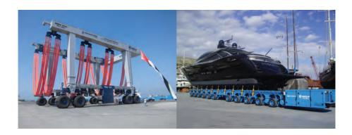
Cimolai Technology Spa supplies customized mobile boat hoists ranging from 30 t to 2000 t diesel and full electric, ship lifting platforms "cimolift" to launch and dry-dock huge vessels, special cranes to move, lift and turn ship blocks, self-propelled modular trailers spmt and transfer systems to support the "cimolift" or to be used independently to perform the transportation and parking operations of the vessels within the shipyards.
