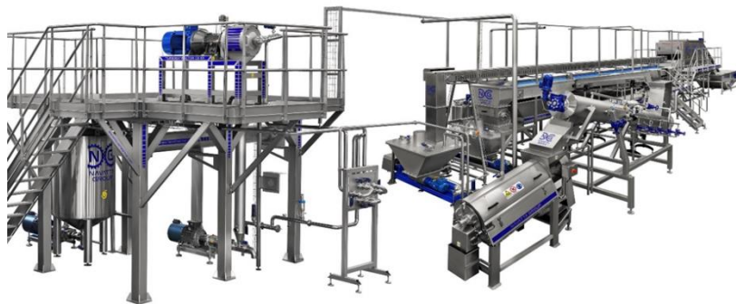
Complete tropical fruit processing line from fruit receiving to pulp extraction
